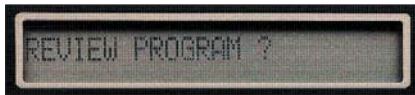
The 900's 24-character alphanumeric display prompts the user through the programming steps.
