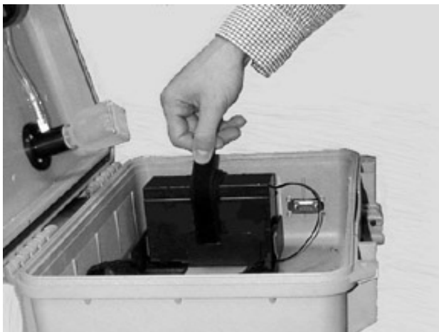
Figure B-12: Tighten Velcro Around Battery.
