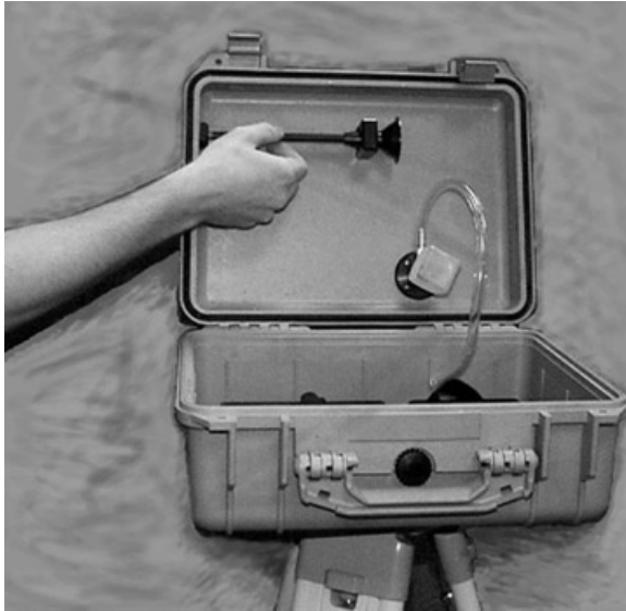
Figure B-3: Unscrew Inlet from Inner Bracket
