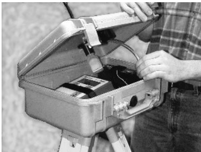
Figure B-10: Keeping the Tube Unkinked
