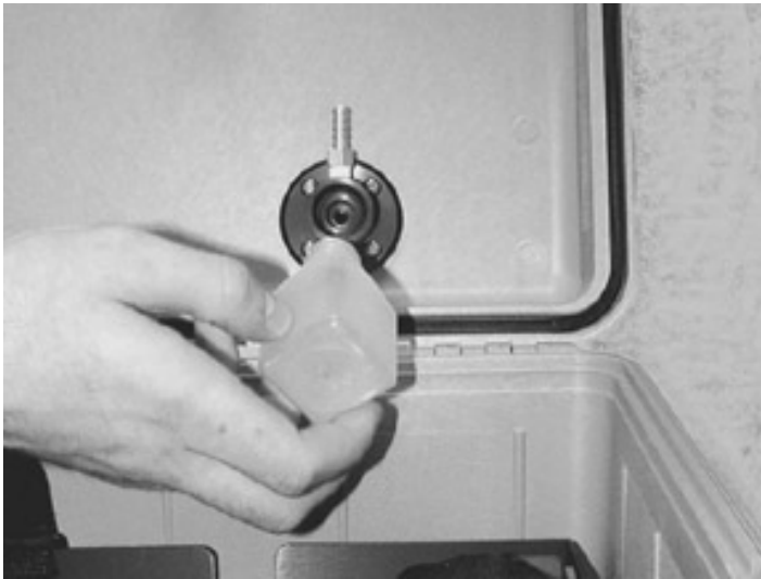
Figure B-5: Installing the Water Trap Bottle
