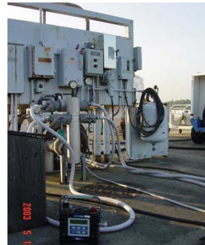
Figure 4. AreaRAE monitoring mechanical equipment.
