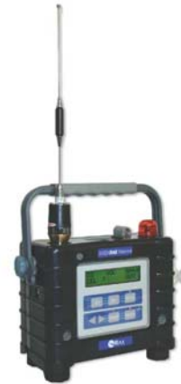
Figure 1. AreaRAE Gamma Wireless Monitor with GPS.
